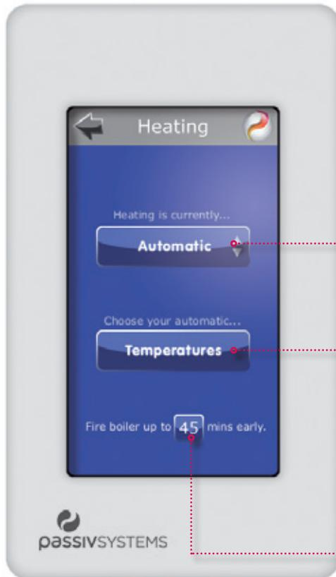
This is where you control how PassivEnergy manages your heating. Don't forget that PassivEnergy runs your heating according to your **OCCUPANCY**, so if you want to control the times your heating is on, you should touch **MENU** then **SCHEDULE** instead.
