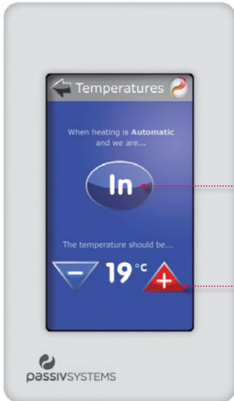
To tell PassivEnergy how warm you normally like to be, touch **MENU** , then **HEATING** , then **TEMPERATURES** .
